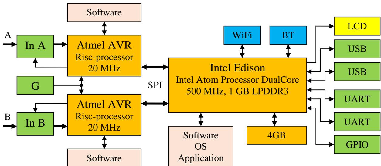
Fig. 1. The block diagram of a microprocessor frequency meter
