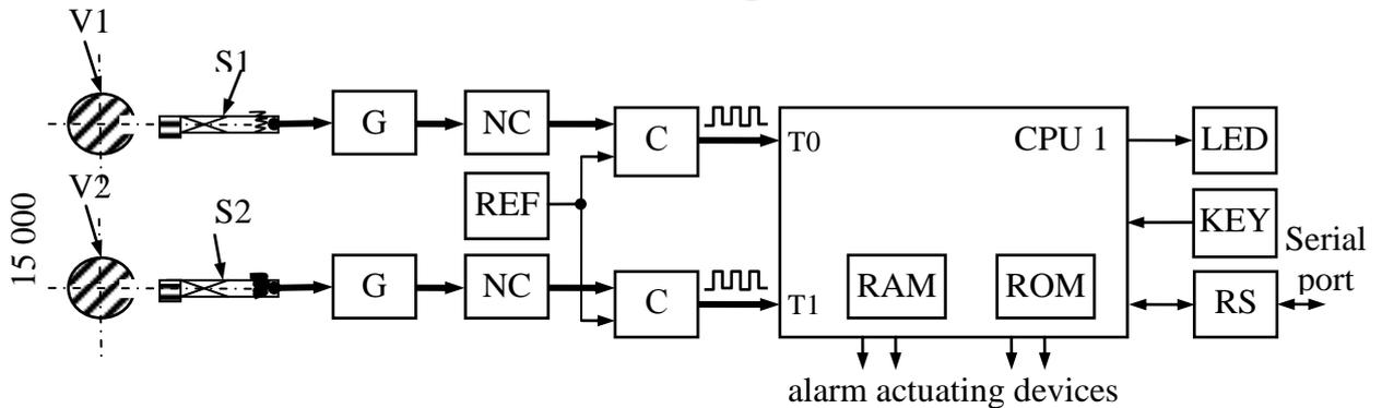
Fig. 1. The block diagram of the measuring channel of the shaft rotational speed
